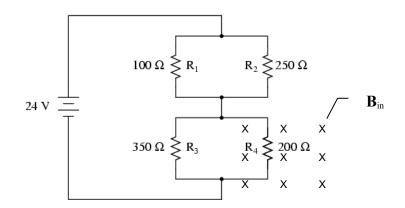
To find the magnetic force, the current through  $R_4$  must be calculated. The two parallel circuit pairs can be replaced with individual resistors:  $R_{1P2} = 71.43 \Omega$  and  $R_{3P4} = 127.27 \Omega$ . These equivalent resistors are now in series, i.e. a voltage-divider configuration. The voltage across the  $R_3$ - $R_4$  combination, which is the voltage across  $R_4$  is
